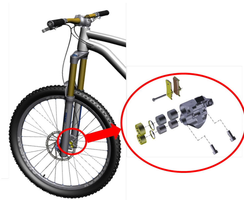
Fig 3 Mountain Bike front brake sub-system: Design details (Sheet 1 of 2)
